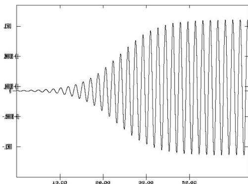
**Figure 3. Amplitude of oscillation vs. time of the numerical model described in reference (7).**
