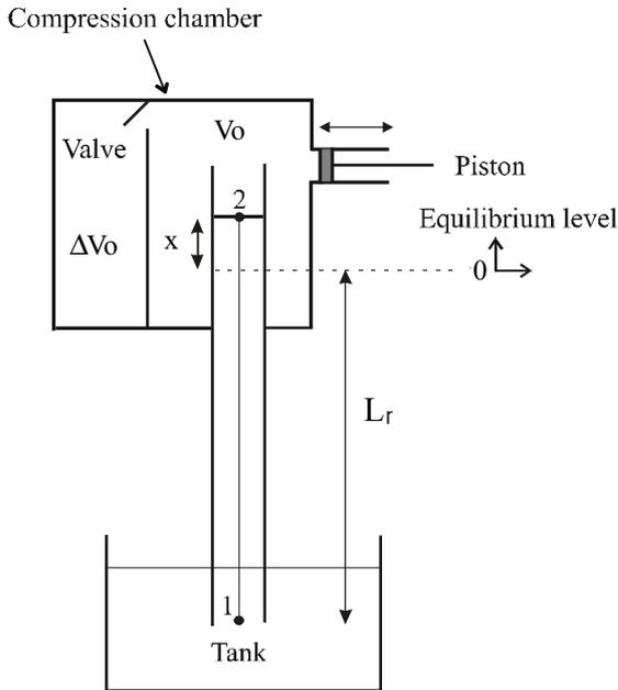
**Figure 1. Schematic diagram of the oscillating water column.**
