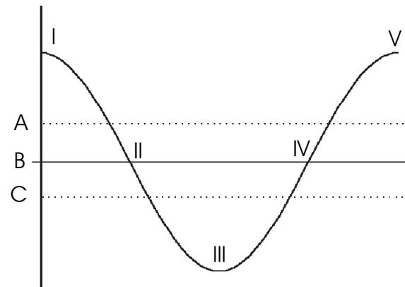
**Figure 4. Water level of the oscillating water column vs. time. Point B represents the reference level.**
